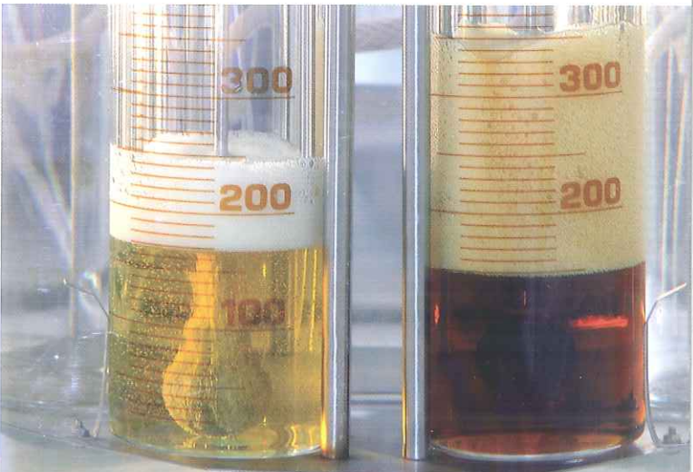
Foam behaviour according to ASTM D 892
